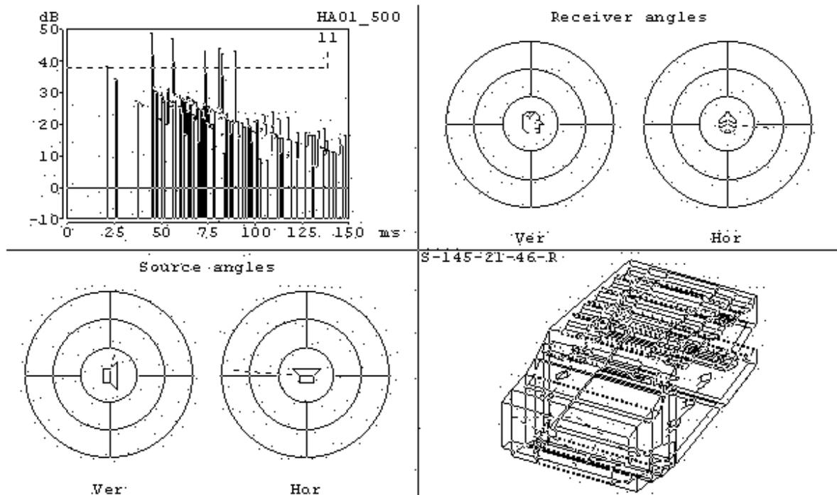
Figure 2 - Echogram and ray tracing for early reflections on a concert hall stage
