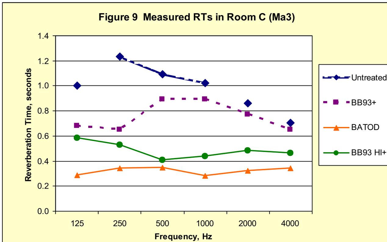
In this room the measured reverberation times in the conditions designed to comply with the BB93 and BB93 HI criteria exceeded those criteria, although to a lesser extent than in Room Ma1. The curves are therefore denoted BB93+ and BB93HI+ on the graph. The results are summarised below.
