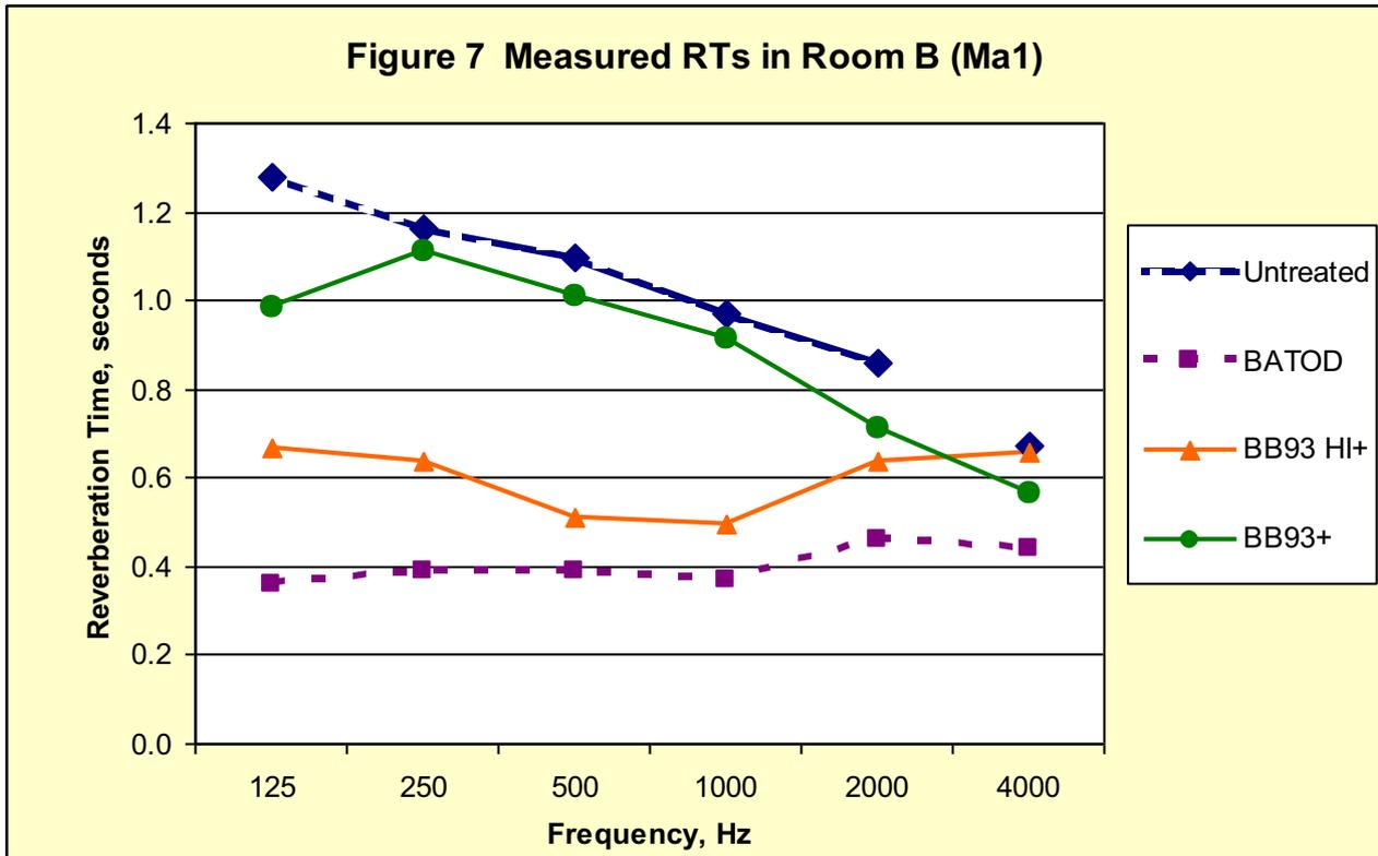
It is not possible to design acoustic absorption in a room to match a reverberation time curve exactly, especially given the need to minimise visual changes to the room and to undertake the changes at weekends. In this case the measured reverberation times in the conditions designed to comply with the BB93 and BB93 HI criteria in fact exceeded those criteria and are therefore denoted BB93+ and BB93HI+ on the graph. The results are summarised below.
