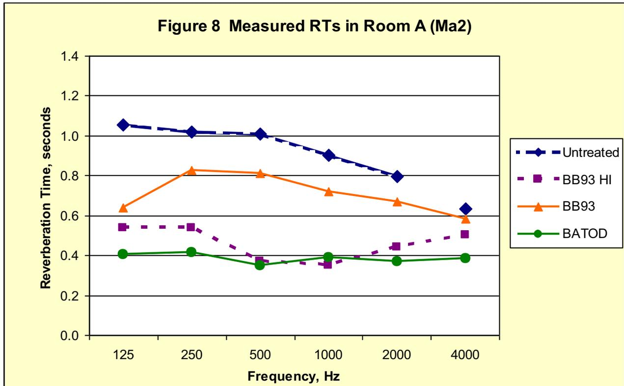
In this room the measured reverberation time in each condition complied with the targets. The results are summarised below.
