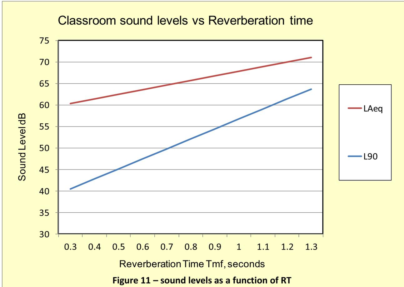
The background noise level LA90 decreased very significantly as the reverberation time reduced. A reduction in reverberation time from 1.2 to 0.8 seconds (that is, from an untreated classroom to one which just complies with the BB93 standard for mainstream secondary classrooms) corresponded to a decrease of 9 dBA in LA90. A further decrease from 0.8 to 0.4 seconds corresponded to a further decrease of 9 dBA. A 9 dBA decrease is very significant, and an 18 dBA decrease is very significant indeed.
