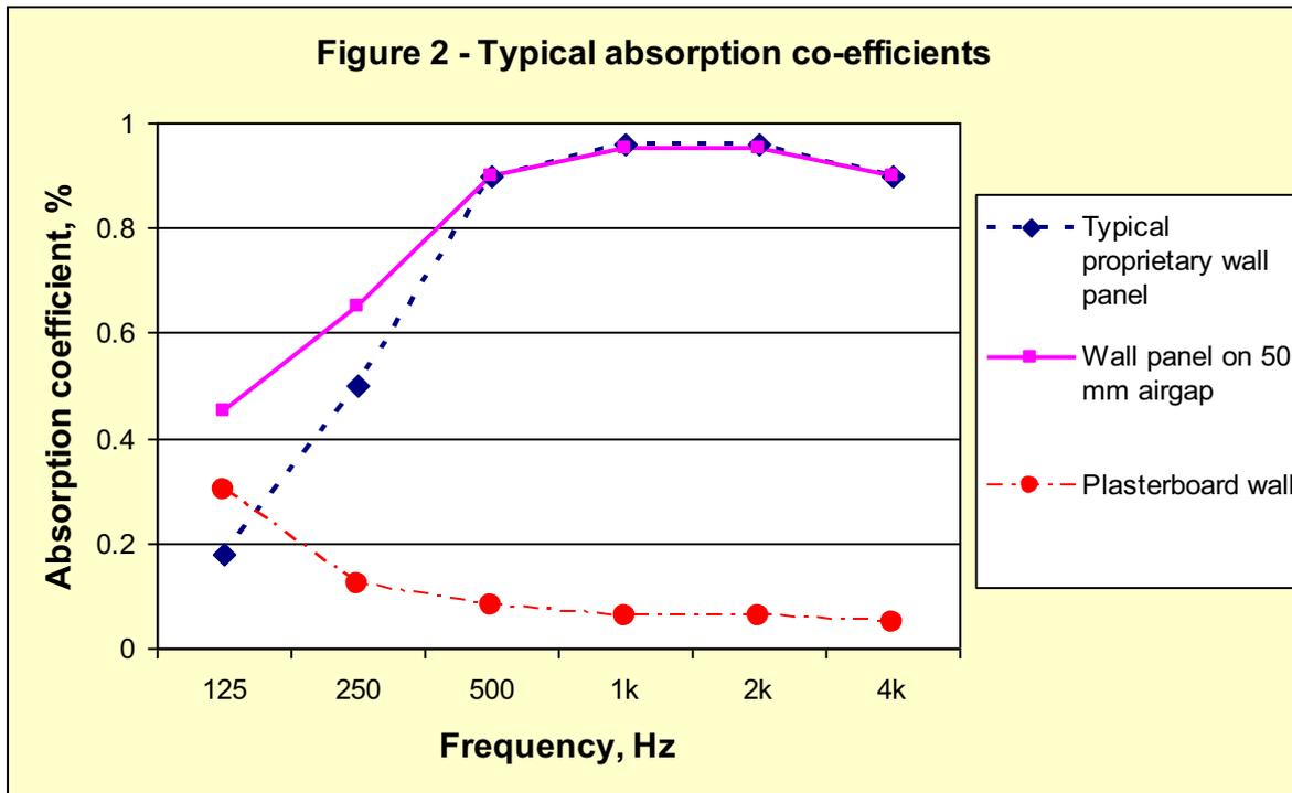
Rooms with masonry walls are naturally more reverberant at low frequencies and reducing this low-frequency reverberation can require large areas of low-frequency absorptive treatment, which typically requires a material over a substantial airgap. With acoustically absorbent ceilings this airgap can be anything up to 200 mm, while with wall panels airgaps of 50 mm are the most that can normally be accommodated.
