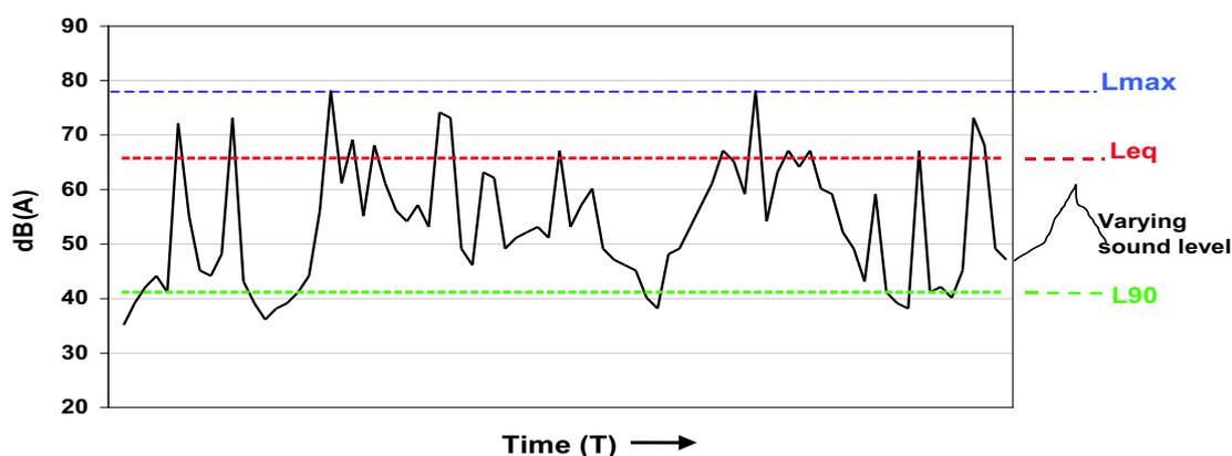
Figure 6 - Time varying sound pressure level
